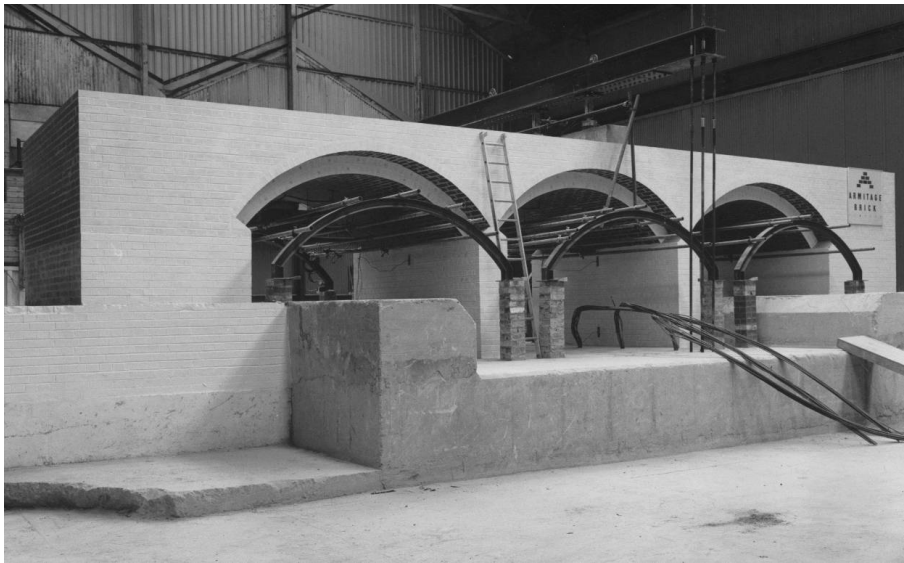
Figure G.2: Bolton bridge Multi-2 built with detached spandrel walls awaiting testing
