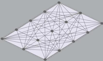
4. Optimization is used to find the layout of discontinuities defining the critical yield-line pattern:
