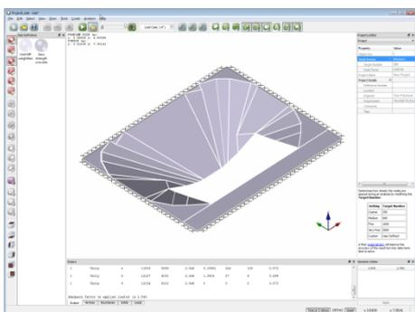
Animated output enables a deeper understanding of slab behaviour at the point of failure to be gained
