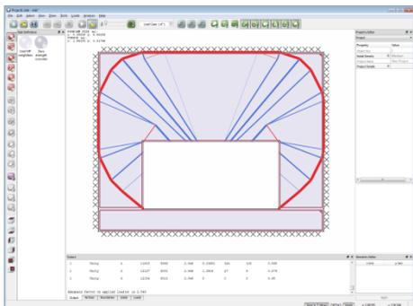
Yield-line theory and optimization technology are combined to allow rapid identification of the critical failure mechanism and associated margin of safety
