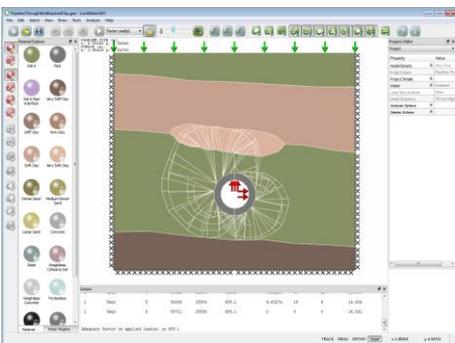
**Modelling a pipeline buried in a multi-layered clay soil**
