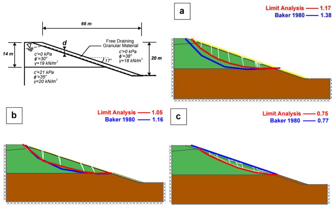
**FIG. 7. Top left) Geometry of slope with free-draining face and comparison of failure surfaces when face is a) 1 m; b) 0.5 m; and c) 0 m.**
