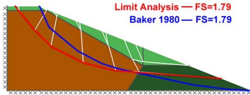
**FIG. 4. Comparison of failure surfaces dam example (nodal spacing=0.7 m).**
