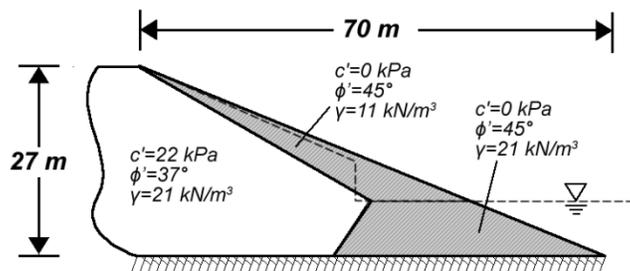
FIG. 3. Original geometry and soil properties of earthen dam.
