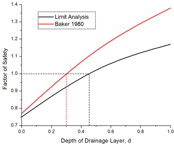
**FIG. 8. Graphical comparison of FS from LA and Baker (1980) over varying drainage depth.**
