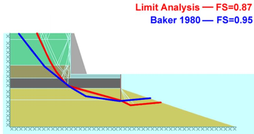
**FIG. 6. Failure surfaces for retaining wall/sheet pile placed on slope.**
