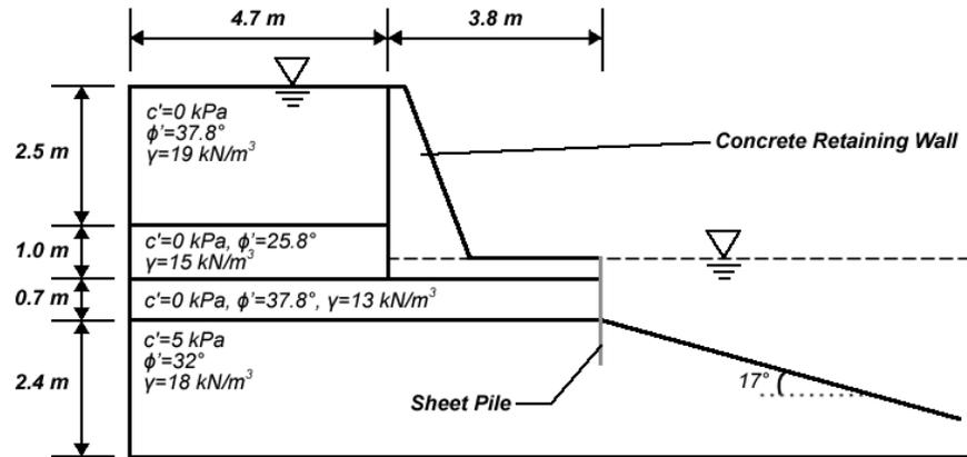
**FIG. 5. Geometry of complex geometry with rapid drawdown.**
