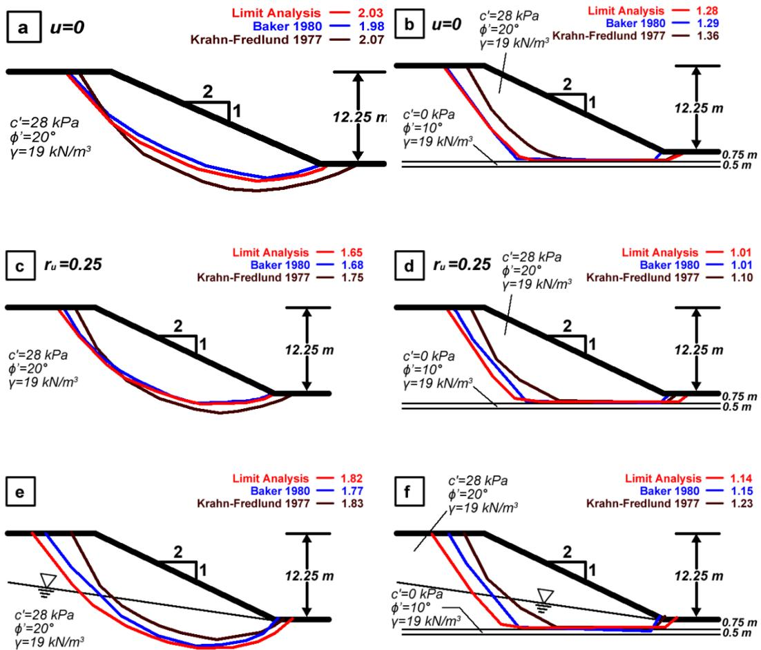
FIG 2. Simple slope analyses a) baseline case; b) underlying weak clay seam with no pore pressure; c) pore pressure,  $r_u=0.25$ ; d) underlying weak clay seam,  $r_u=0.25$ ; e) no clay seam, sloped water table; f) clay seam, sloped water table.
