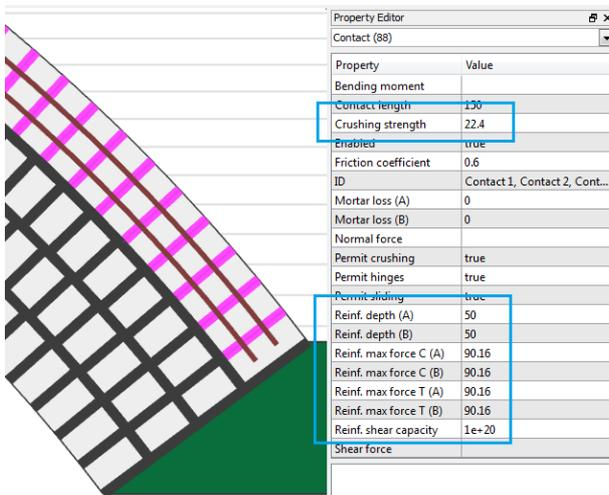
Figure 3: Saddle - general Contact properties
