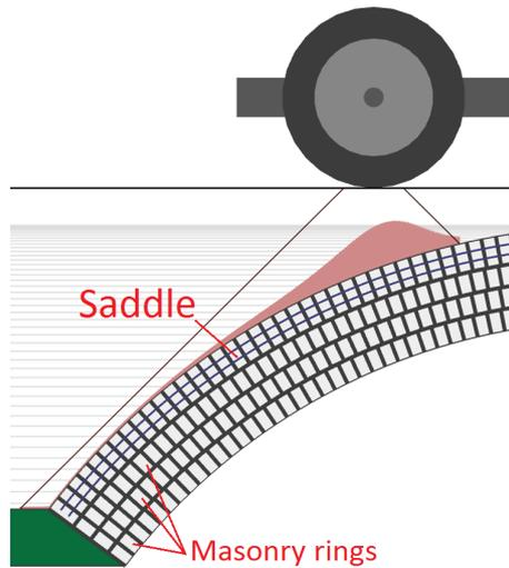
Figure 2: TRL 3-ring arch with saddle, as modelled in LimitState:RING
