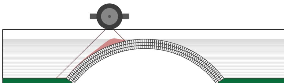
Figure 1: TRL benchmark 3-ring arch, as modelled in LimitState:RING
