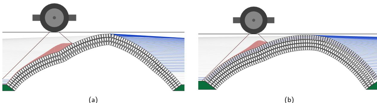
Figure 5: LimitState:RING critical failure mechanisms: (a) unreinforced, and (b) saddled TRL arch bridges
