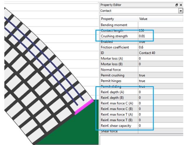
Figure 4: Saddle - end Contact properties
